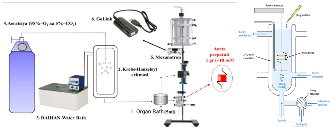
Fig. 1 A schematic diagram of the setup used to control and measure the isometric contraction of isolated rat aortic smooth muscle is shown. (1) The organ bath (5 mL) is connected to a dedicated reservoir that circulates the solution. (2) The Krebs-Hanseleyt eritmasi solution is used to maintain physiological conditions. (3) A thermostat regulates the temperature to ensure it remains constant and within the physiological range. (4) The
